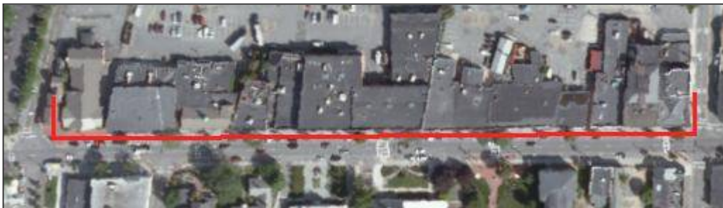
◀ On Main Street between Barnstable Rd. and Winter St., all buildings have a consistent ground-floor façade. New infill development should maintain or help create a consistent setback line.
